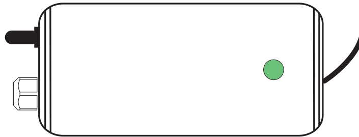
Green LED indicates UV lamp “ON”.
